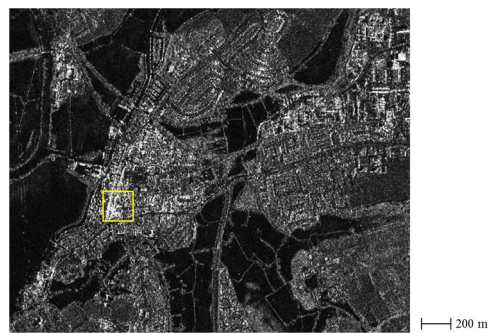
Fig. 16 TerraSAR-X image showing flooding in the urban areas of Tewkesbury in July 2007 (pixel intensities are DN backscatter values, dark areas are water, 2.6 \times 2 km, © DLR). Yellow rectangle covers unflooded urban area sample.
