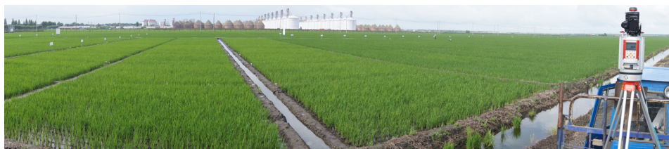
Fig. 2 Overview of the investigated field experiment from scan position six (Fig. 3). On the right side the scanner with the tripod mounted on the small trailer can be seen (taken: July 4, 2011).
