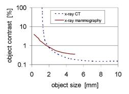
**Fig. 5** Contrast-detail curves showing the values for a mammography system and for a CT system, illustrating the inherent strengths and weaknesses of each system. The mammography system is strongest for imaging smaller objects, below 2 mm diam, as lower contrasts can be detected. In comparison, CT cannot image objects smaller than 1 mm, but can image subtle changes in contrast better when the objects are larger than 2 mm.
