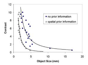
**Fig. 8** Contrast-detail analysis of diffuse imaging with and without *a priori* information about the fat and fibroglandular layer of the breast, estimating the detectable levels of contrast for given object sizes. With the inclusion of *a priori* fat/glandular tissue layers, the minimum contrast required for each size is decreased to achieve the same CNR value.
