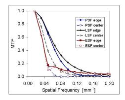
**Fig. 3** MTF profiles of the graphs shown in Fig. 2, illustrating the information contained as a function of spatial frequency, with LSF having highest resolution, PSF having next highest, and ESF having the lowest. Resolution is always considerably worse in the interior of the diffusing medium than at the edge near a source or detector.
