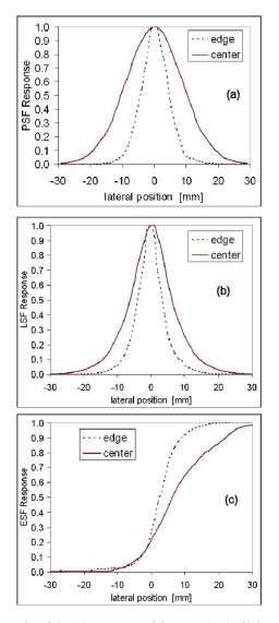
**Fig. 2** Graphs of the (a) point spread function (PSF), (b) line spread function (LSF), and (c) edge spread function (ESF) for "pencil-beam" transmission through a 60-mm slab, having diffuse interaction coefficients of  $\mu_a$ =0.01 mm<sup>-1</sup>  $\mu'_s$ =1.0 mm<sup>-1</sup>. In all three cases, two locations were analyzed using a target near the edge (2 mm inside the surface) and then at the center of the slab.
