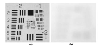
**Fig. 1** Images of the USAF test field, imaged (a) through air and (b) through 2 mm of 1% intralipid solution. The ability to use this type of resolution tool in a diffusing medium is very limited.
