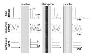
**Fig. 6** Time-domain, frequency-domain, and continuous wave measurement sensitivities to absorption and scatter. Schematic shows simplistically how absorbing and scattering structures will change TD and FD data, but that in transmission, their effect on cw data will be indistinguishable.
