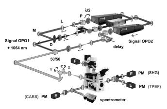
**Fig. 5** CRS with two OPOs. F and E stand for Forward and Epi (backward) detection; PM for photomultiplier tubes; M for silver mirrors; P for polarizer, and L for NIR achromatic doublets.
