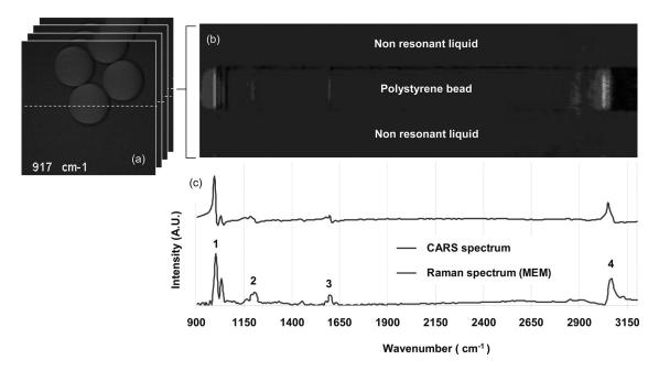
**Fig. 9** Hyperspectral imaging of 20- $\mu$ m polystyrene beads. (a) Image at 917 cm<sup>-1</sup> (NRB); (b) hyperspectral section of a single bead versus Raman shift; and (c) recorded CARS spectrum of the bead (upper curve) and processed with the maximum entropy method (MEM) (lower curve). Recovered Raman peaks 1: 1003 and 1033 cm<sup>-1</sup>; 2: 1158 and 1188 cm<sup>-1</sup>; 3: 1584 and 1604 cm<sup>-1</sup>; and 4: 3065 cm<sup>-1</sup> Stokes and pump powers were 15 mW.
