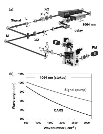
**Fig. 3** (a) Efficient CARS setup using one OPO. The fundamental 1064nm and OPO signal pulse trains are recombined and used as the pump and Stokes beams, respectively. F and E stand for Forward and Epi detection; PM for photomultiplier tubes; M for silver mirrors; P for polarizer, and L for NIR achromatic doublets. (b) Fundamental 1064nm, OPO signal, and anti-Stokes CARS associated with the various Raman shift.
