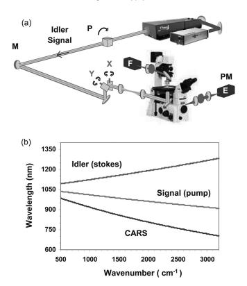
**Fig. 1** (a) Simplest CARS setup using one OPO. The signal and idler trains are collinear, overlapped in time, and used as the pump and Stokes wavelengths, respectively. F and E stand for Forward and Epi (backward) detection; PM for photomultiplier tubes; M for silver mirrors, and P for polarizer. (b) Signal, idler, and anti-Stokes CARS wavelengths associated with the various Raman shift.
