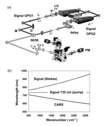
**Fig. 8** Using two OPOs for hyperspectral imaging. (a) Scheme of the experiment where the two OPO signals are used. F and E stand for Forward and Epi (backward) detection; PM for photomultiplier tubes; M for silver mirrors; P for polarizer; L for NIR achromatic doublets, and D for dichroic filter. (b) OPOI set at 735 nm (pump), OPO2 signal (Stokes) and anti-Stokes CARS wavelengths associated to Raman shifts.
