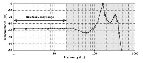
Fig. 5 Frequency response of the measurement system.
