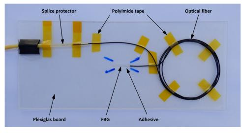
Fig. 2 Construction of the sensor.
