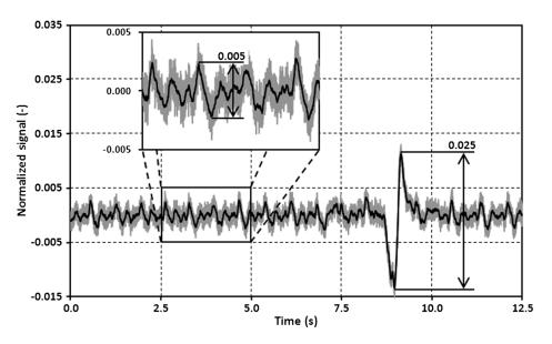
Fig. 16 Signal artifact caused by a short displacement of the track table.
