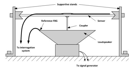
Fig. 4 Setup for determining the system's frequency response.
