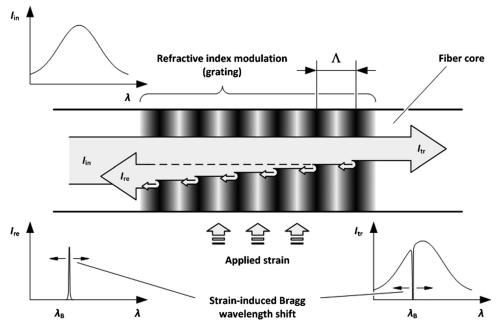
Fig. 1 Principle of operation of an FBG.
