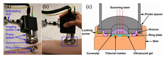
**Fig. 1** PS-OCT imaging interface for coupling the imaging probe and the skin. (a) and (b) Photographs of the imaging interface before and after coupling the imaging probe and the skin. (c) A magnified sketch of the probe spacer and ring plate, corresponding to the region in (b) delineated by the dashed blue rectangle.
