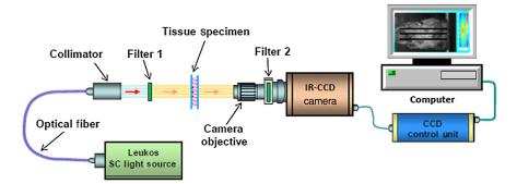
**Fig. 1** Optical setup for optical imaging of tissue using selective filters 1 and 2 (1200 nm narrow-band and 1500 nm longpass) and wavelengths from the second and third windows from the Leukos supercontinuum (SC) light source.
