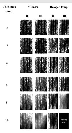
Fig. 2 Images of chicken tissue at various thicknesses (from  $\sim$ 2 to 10 mm) and three wires from the SC laser and halogen lamp light sources, using wavelengths from the second (II) and third (III) optical windows.
