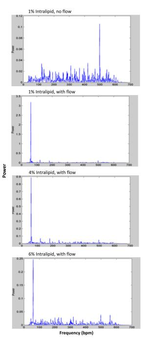
**Fig. 7** Power spectra calculated from single-point data collected from varying tissue phantoms using the PPG imager.
