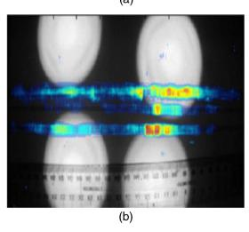
**Fig. 8** PPG images taken at two distances from the bare-vessel phantoms to assess spatial resolution [(a) 10 cm and (b) 20 cm]. At all test distances, the PPG imager was able to detect flow patterns between tubes placed 5 and 10 mm apart but not between the tubes placed only 1 mm apart. At the 20-cm test distance, the PPG imager did not maintain this level of resolution along the periphery of its field of view.
