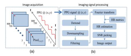
**Fig. 2** Time-resolved PPG signal extraction. (a) Intensity at image pixel (x, y) is extracted sequentially from 800 contingent frames. (b) Processing method for quantifying PPG signals.
