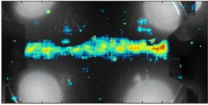
Fig. 6 Flow images of the tissue phantom collected with the PPG imager. Test conditions are labeled above each pair of images. Flow was established at 60 bpm.
