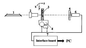
Fig. 3 Experimental setup for in vitro studies of optical clearing of tissue samples. 1—single-mode He-Ne laser; 2—microscope objective; 3-glass cuvette with studied specimen embedded in Trazograph solution; 4—scanning device; 5—manually rotating polarizer; 6—photomultiplier tube with pinhole; 7—control and data acquisition system.
