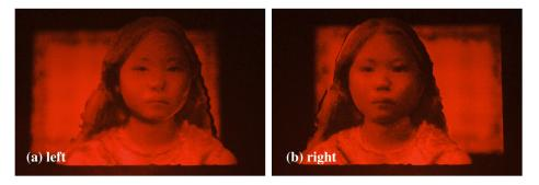
Fig. 13 Optical reconstruction of the polygon-based high-definition computer hologram named "Shion" by using transmitted illumination of a He-Ne laser (Video 2, WMV, 8.8 MB). The polygon-modeled object is rendered by texture mapping and Gouraud shading. Photographs (a) and (b) are taken from different viewpoints.
