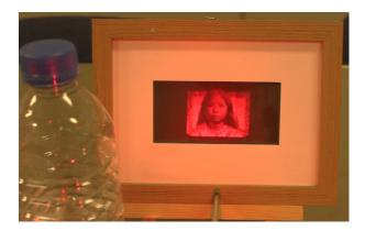
Fig. 14 Optical reconstruction of "Shion" by using an ordinary red LED (Video 3, WMV, 10.8 MB).
