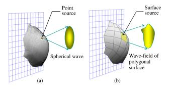
Fig. 1 Schematic comparison of the point-based method (a) and polygon-based method (b).
