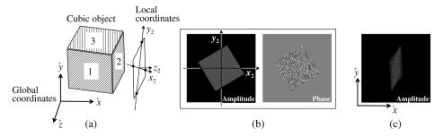
Fig. 3 An example of surface functions (b) for polygon 2 of a cubic object (a). The amplitude image of the polygon field (c) after rotational transform agrees with the shape of the original polygon.
