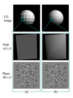
Fig. 7 Examples of the surface function for flat shading (a) and Gouraud shading (b).
