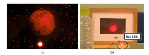
Fig. 11 Optical reconstruction of "The Moon" by using transmitted illumination of a He-Ne laser (a) and reflected illumination of an ordinary red LED (b) (Video 1, WMV, 7.8 MB). The sphere object is rendered using texture mapping and flat shading.
