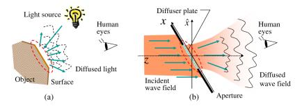
Fig. 2 Theoretical model of polygonal surface sources of light (b) that imitate the surface of an object (a).
