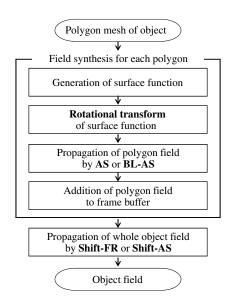
Fig. 4 Numerical procedure for computing entire object fields.
