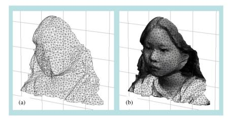
Fig. 12 Polygon mesh of a live face whose shape is measured using a 3D laser scanner (a), and its rendering with CG using texture mapping.
