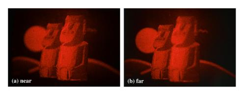
Fig. 6 Photographs of the optical reconstruction of a polygon-based high-definition computer hologram named "Moai II".<sup>2</sup> The camera is focused on the near moai (a) and far moai (b).
