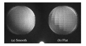
Fig. 8 Simulated reconstruction of spheres rendered by Gouraud shading (a) and flat shading (b).
