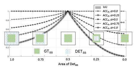
**Fig. 9** Analysis of ACC<sub>*R*</sub>. GT<sub>BB</sub> is fixed at 50% of input image volume, and  $Det_{BB}$  goes from maximum FP to maximum FN from left to right.
