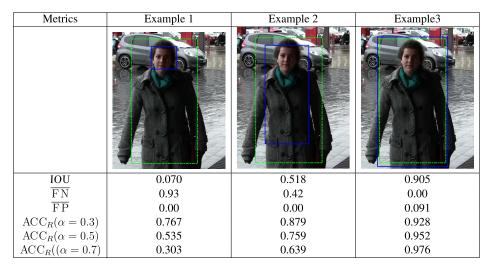
**Fig. 10** Comparison of IOU and ACC<sub>R</sub> with varying values of  $\alpha$ . Solid blue line is detected bounding box and dashed green line is ground truth bounding box. Example image from PEVid dataset.<sup>30</sup>
