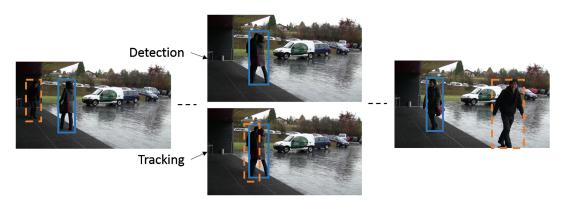
**Fig. 4** Illustration of object detection compared with object tracking for a video stream. In the case of occlusions (center), tracking techniques are able to project the location of the object using temporal information. Example video from PEVid dataset.<sup>30</sup>
