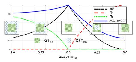
**Fig. 8** Comparison of IOU,  $\overline{FN}$ ,  $\overline{FP}$ , and  $ACC_R$ .  $GT_{BB}$  is fixed at 50% of input image volume, and  $Det_{BB}$  goes from maximum  $\overline{FP}$  to maximum  $\overline{FN}$  from left to right.
