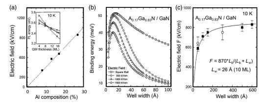
**Fig. 11** (a) Built-in electric field as a function of Al composition in AlGaN/GaN quantum well structure. Reproduced with permission from Ref. 111. (b) Calculated binding energy in AlGaN/GaN structure versus GaN well thickness at different electric fields. (c) The electric field as a function of barrier thickness for the same structure as Fig. 11(b). Reproduced with permission from Ref. 112.
