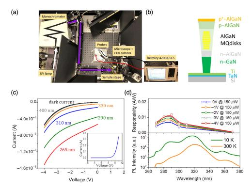
**Fig. 20** (a) The setup for responsivity measurement. (b) The structure of AlGaN-based NWs grown on Ti/TaN/Si. (c) Reverse bias current versus voltage curves at the different excitation wavelengths. The inset shows the forward bias current versus voltage curve. (d) Responsivity spectra with 0.5 mW/cm² lamp excitation and photoluminescence spectra.
