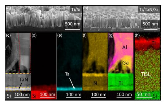
**Fig. 6** (a) and (b) SEM images showing the NWs/substrate interface roughness comparison between the sample on Ti/Si and Ti/TaN/Si. (c)–(g) Dark-field cross-sectional TEM images and EDX elemental mapping of the sample on Ti/TaN/Si substrate. (h) Electron energy loss spectroscopy mapping of the sample on Ti/Si showing the interdiffusion and  $TiSi_x$  formation, leading to the rough surface. Reproduced with permission from Ref. 42.
