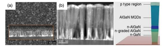
**Fig. 9** (a) Top-view of SEM image and tilted-view (inset) of NWs-LED. (b) Cross-sectional high angle annual dark-field scanning transmission electron microscopy (HAADF-STEM) scan showing p-i-n AlGaN NWs with coalesced p-GaN contact layer and 15 pairs of Al<sub>0.3</sub>Ga<sub>0.7</sub>N/Al<sub>0.5</sub>Ga<sub>0.5</sub>N quantum disks/quantum barriers (left) along with a schematic representation of the layer structure (right). Reproduced with permission from Ref. 48.
