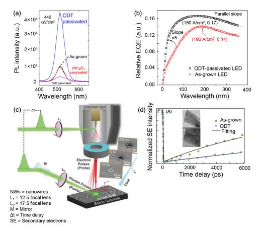
**Fig. 15** ODT surface passivation of InGaN/GaN NWs showing enhanced (a) photoluminescence and (b) EQE. Reproduced with permission from Ref. 64. (c) Schematic of 4D S-UEM set-up schematic and (d) SE intensity improvement for the ODT-passivated InGaN NWs. The inset shows the SEM image of carbon deposition at the NW sidewall. Reproduced with permission from Refs. 141 and 142.
