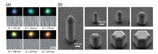
**Fig. 7** (a) Tilted-view of SEM and emission images from SAG InGaN/GaN NWs as a function of different nanohole diameters. Reproduced with permission from Ref. 82. (b) Tilted-view of SEM images from InGaN/GaN single NW having various diameters. Reproduced with permission from Ref. 50.
