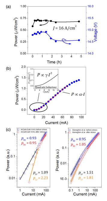
**Fig. 18** AlGaN/GaN NWs-LED reliability test. (a) Power (*Y*-axis) and voltage (alternate *Y*-axis) versus time plot at low-injection current. (b) Power–current characteristic of the device after stress test showing the low- and high-injection current regimes. (c) Semilog plot of power versus current comparing characteristics of NWs and planar devices. Reproduced with permission from Ref. 48.
