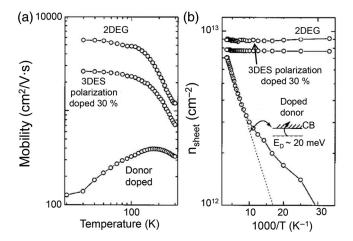
**Fig. 13** The temperature-dependent (a) mobility and (b) carrier sheet densities for a polarization-doped sample of 3DES, donor-doped sample, and a 2DEG sample structures. Reproduced with permission from Ref. 13.
