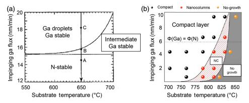
**Fig. 1** (a) Surface structure diagram of GaN growth depicting the Ga flux ( $\Phi_{Ga}$ ) conditions plotted versus growth temperature for a constant *N*-flux ( $\Phi_N$ ) of 15.2 nm/min. Reproduced with permission from Ref. 56. (b) Growth diagram showing the growth conditions-dependent surface morphology of GaN/Si(111) as a function of  $\Phi_{Ga}$  and growth temperature for constant  $\Phi_N$  (6.0 nm/min). Reproduced with permission from Ref. 55.
