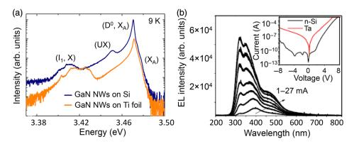
**Fig. 8** (a) Low-temperature photoluminescence spectra of GaN NWs grown on Ti foil. Reproduced with permission from Ref. 83. (b) Electroluminescence spectra from AlGaN-based UV NWs-LEDs on flexible Ta foil; inset shows current-voltage characteristics of LEDs on Ta foil (red) and Si substrate (black). Reproduced with permission from Ref. 39.
