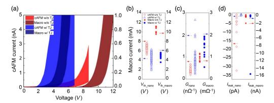
**Fig. 17** cAFM measurement for graded AlGaN NWs: (a) current versus voltage curves, (b) comparison of nanoscale and macroscale turn-on or threshold voltages ( $V_{th\_nano}$  or  $V_{th\_macro}$ ), (c) comparison of nanoscale and macroscale differential conductance ( $G_{nano}$  or  $G_{macro}$ ), and (d) leakage current at -1 V ( $I_{leak\_nano}$  or  $I_{leak\_macro}$ ). Reproduced with permission from Ref. 167.
