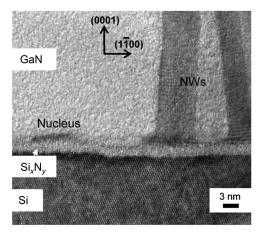
**Fig. 2** Cross-sectional view of high-resolution transmission electron microscopy (TEM) image of GaN NWs on Si(111) showing the formation of the interfacial amorphous  $Si_xN_y$  interlayer. Reproduced with permission from Ref. 69.
