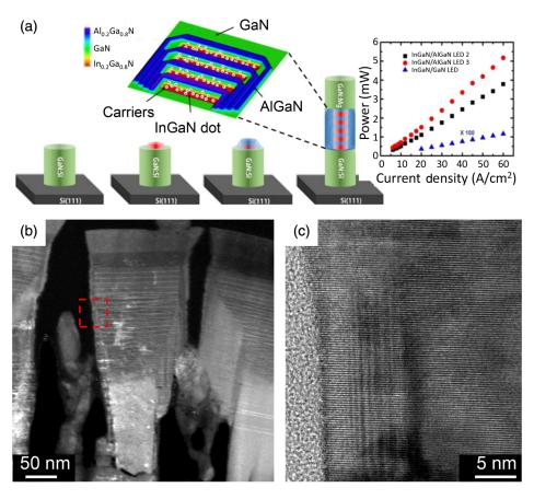
**Fig. 16** (a) InGaN/GaN growth schematic with AlGaN core—shell layer and output power enhancement. Reproduced with permission from Ref. 155. (b) HAADF-STEM of AlGaN-based p—i—n NW structures on Ti (500 nm)/Mo substrate. (c) Active region showing multiple AlGaN shells surrounding 15 stacks of uniform quantum disks/quantum barriers.
