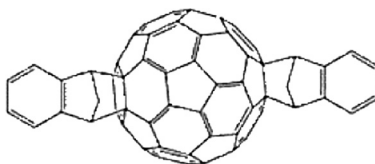
Fig. 4 Molecular structure of indene-C 60 bis-adduct.
