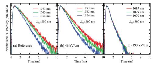
**Fig. 4** Detection wavelength dependence of PL decay profile measured at 3 K for (a) a reference sample and SCs at (b) 46 and (c) 193 kV/cm. The excitation laser wavelength was 800 nm, which provides excitation above the GaAs barrier. The excitation powers for (a), (b), and (c) were 100, 100, and 250  $\mu$ W, respectively. Reprinted with permission from Ref. 50. © 2014 AIP Publishing LLC.
