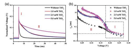
**Fig. 18** (a) Normalized open-circuit photovoltage decay curves for bulk heterojunction ZnO/PbS QDHSCs with and without the  $TiO_2$  coating on the ZnO-NWs, showing two dominant decay processes, I and II. (b) The effective carrier lifetime calculated from the voltage decay curves.<sup>139</sup>
