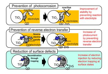
**Fig. 12** Schematic illustration of the effects of surface passivation on QD adsorbed photoelectrodes in QD sensitized solar cells: (1) prevention of photocorrosion; (2) prevention of reverse electron transfer; and (3) reduction of surface trap states.
