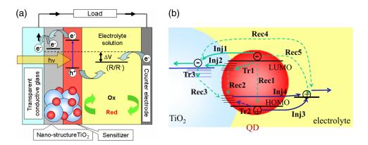
**Fig. 11** Schematic illustrations of (a) the working principle and configuration of QD-sensitized solar cells and (b) possible charge transfer processes occurring at TiO<sub>2</sub>/QD/electrolyte interfaces, including injection (Inj), trapping (Trp), and recombination (Rec) of photoexcited carriers.
