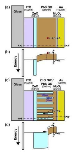
**Fig. 16** (a) Schematic and (b) energy band diagram at short-circuit (cross-section along A-A') of a planar depleted heterojunction QDHSC, and (c) schematic and (d) energy band diagram (cross-section along B-B') of a bulk heterojunction QDHSC. Reprinted with permission from Ref. 135. © 2013 by John Wiley Sons.
