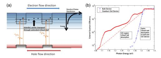
**Fig. 9** (a) Schematics of proposed interdot carrier transfer mechanism through continuum density of states due to Urbach tail absorption in the GaAs matrix intrinsic layer and (b) EQE of GaAs/InAs QD sample with no antireflection coating. The Urbach tail contributions for both devices are shown by the dotted lines. Reprinted with permission from Ref. 73. © 2013 AIP Publishing LLC.
