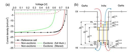
**Fig. 3** (a) Energy band model of the InAs/GaAs system, as considered in this work. (b) J - V characteristics of nonexcitonic and excitonic QDSCs, simulated under full (solid lines) and filtered ( $\lambda > 870$  nm, dashed lines) AM1.5G solar spectrum illumination. The additive feature of the QD contribution can be inferred by observing the reference cell and QDSCs currents at short circuit. Reprinted with permission from Ref. 46. © 2016 IOP Publishing.
