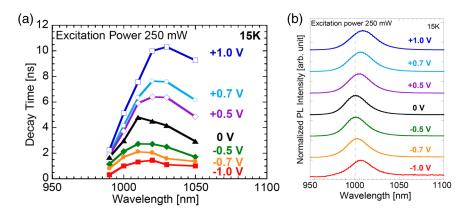
**Fig. 5** (a) Relationships between PL decay time spectra and bias voltage. Ultrahigh density InAs QDs with 2.2 mL was inserted into GaAs pn-junction. (b) PL spectra of ultrahigh density InAs QDs with 2.2 mL as a function of bias voltage. Reprinted with permission from Ref. 54. © 2013 IEEE Publishing.
