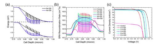
**Fig. 6** (a) APSYS modeled band diagram for  $0e^{-}/QD$  (black) and  $4e^{-}/QD$  (blue) structures in the dark at 0 V applied bias. (b) APSYS modeled SRH rates at 1.0-V applied bias across the i-region of varying delta-doping levels. (c) Measured 1-Sun AMO J - V characteristics of devices. Reprinted with permission from Ref. 61. © 2014 IEEE Publishing.
