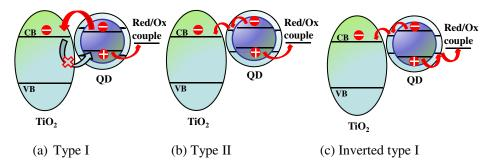
Fig. 14 Schematic illustration of the structures of core/shell QDs: (a) type I, (b) type II, and (c) inverted type I.
