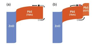
**Fig. 17** Schematic illustration of the proposed band bending at short-circuit conditions in the (a) ZnO/PbS-TBAI and (b) ZnO/PbS-TBAI/PbS-EDT (TBAI = tetrabutylammonium iodide). Reprinted with permission from Ref. 151. © 2014 Nature Publishing Group.
