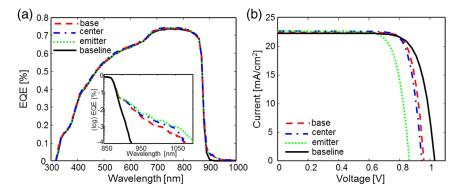
**Fig. 8** (a) Measured EQE versus wavelength. (b) Measured current–voltage characteristics for baseline and QD-enhanced pin-GaAs solar cells. The inset highlights the sub-bandgap photoresponse due to absorption by the QD superlattice. Reprinted with permission from Ref. 69. © 2014 AIP Publishing LLC.
