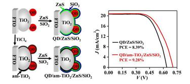
**Fig. 13** An improved surface passivation on photoelectrode with an amorphous  $TiO_2$  (am-TiO<sub>2</sub>)/ZnS/SiO<sub>2</sub> and the PCE of  $CdSe_xTe_{1-x}$  QDSSCs was improved to 9.28%. Reprinted with permission from Ref. 116. © 2015, American Chemical Society.
