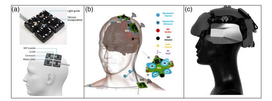
**Fig. 2** Mobile, modular, and wearable fNIRS systems. (a) A wearable fNIRS device consisting of DOT modules for modular design. Adapted with permission from Ref. 45. (b) A device that allows for simultaneous recording of fNIRS, EEG, and other physiological signals. Adapted with permission from Ref. 72. (c) A time-domain fNIRS device with a miniaturized design and whole-head coverage. Adapted with permission from Ref. 73.
