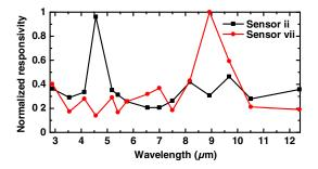
Fig. 4 Measured spectral responsivities for sensors (ii) and (vii).
