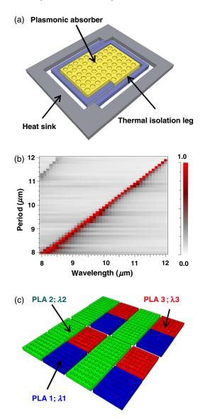
**Fig. 1** (a) Schematic diagram of the uncooled IR sensor (thermopile) with Au-based two-dimensional plasmonic absorber (2-D PLA). (b) Calculated wavelength absorption results for the 2-D PLA as a function of the period. (c) Concept of the pixel array with various 2-D PLAs for multispectral imaging.
