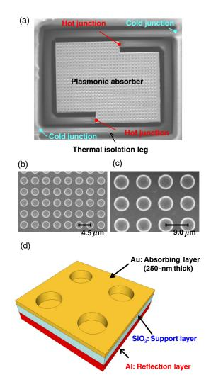
Fig. 3 (a) Scanning electron microscopy (SEM) image of the microelectromechanical system-based thermopile with 2-D PLA developed in this study. Magnified SEM images of the 2-D PLAs of sensors (b) (ii) and (c) (vii). (d) Schematic diagram of the 2-D PLA.
