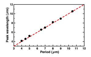
Fig. 6 Peak wavelength of the responsivity as a function of the 2-D PLA surface period.
