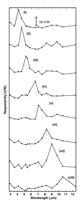
Fig. 5 Spectral responsivity (MWIR and LWIR) for sensors (i)-(viii).
