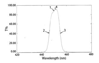
Fig. 11 The transmission spectrum of the 450-nm bandpass filter.
