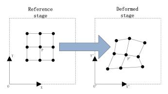
Fig. 19 Strain calculated using points.
