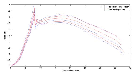
Fig. 4 The comparison of a tensile test at room temperature of speckled and unspeckled specimens.
