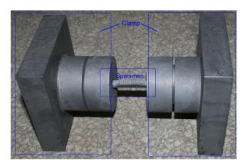
Fig. 25 Specimen before heating.
