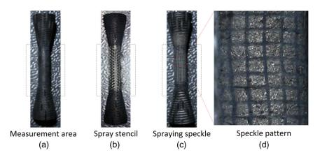
Fig. 2 Specimen. (a) Measurement area located inside of the dashed rectangle. (b) Stencil of spraying placed on the specimen. (c) Speckle pattern after spraying. (d) Speckle pattern on specimen.
