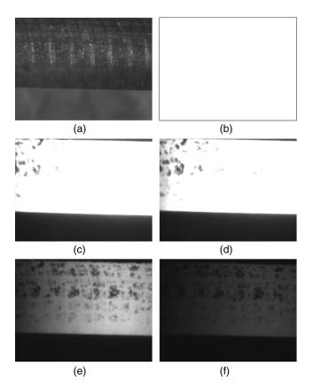
**Fig. 12** Image of a specimen (a) acquired at room temperature; (b) acquired without filter at 2600°C; (c) acquired with one linear polarizing (PL) filter at 2600°C; (d) acquired with one 450-nm bandpass and one PL filter at 2600°C; (e) acquired with two ND8 filters, one 450-nm bandpass filter, and one PL filter at 2600°C; (f) acquired with two ND8 filters, one PL filter, one ND2 filter, one ND4 filter, and one 450-nm bandpass filter at 2600°C.
