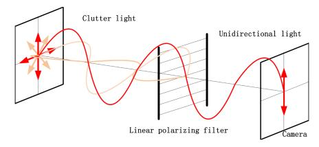
Fig. 14 Linear polarizing filter.
