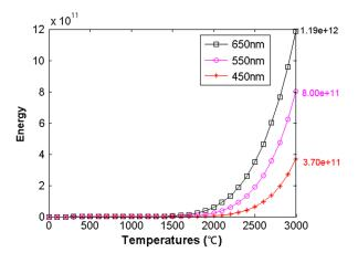
Fig. 8 Thermal radiation energy as a function of temperature for optical wavelength of 450, 550, and 650 nm.
