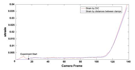
Fig. 27 Digital image correlation result compared with displacement of clamps.
