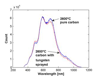
**Fig. 16** Spectra of carbon fiber specimens not sprayed with tungsten and carbon fiber specimens sprayed with tungsten at 2600°C.
