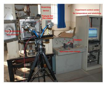
Fig. 22 Heating and stretching devices.
