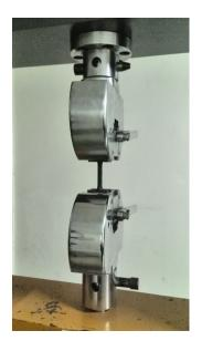
Fig. 3 The tensile test at room temperature of speckled and unspeckled specimens.
