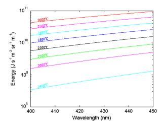
Fig. 7 Thermal radiation energy as a function of wavelength at various temperatures.
