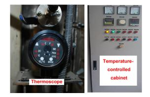
Fig. 21 Temperature measurement and control components for the closed-loop control of temperature.
