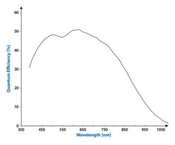
Fig. 6 Quantum efficiency of the CMOS camera used for recording experimental images.
