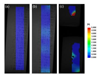
Fig. 28 Strain field of the specimen during stretching.
