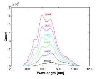
Fig. 10 Spectra of carbon fiber specimens sprayed with tungsten at different temperatures.
