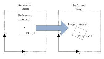
Fig. 18 The basic principle of digital image correlation.
