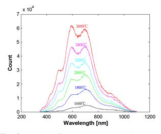
Fig. 9 Spectra of carbon fiber specimens not sprayed with tungsten at different temperatures.
