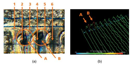
Fig. 12 Occurrence of overheated melt pool on sample (a) and in the temperature map (b).
