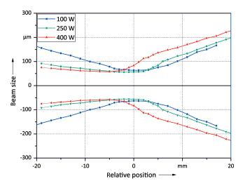
Fig. 7 Caustic of the laser at different power levels.
