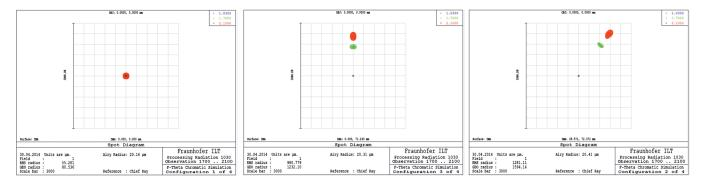
Fig. 5 Displacement of the chief rays for different wavelengths and deflection angles relative to the 1030 nm chief ray (1030 nm in blue, 1700 nm in green, and 2100 nm in red).
