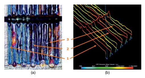
Fig. 11 Sample with remolten metal surface (a) and temperature map (b), processing parameters: laser power 200 W, track width 200  $\mu$ m, feed rate 400 mm/s.
