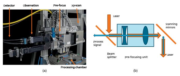
Fig. 2 Optical train with sensor system (a) and sketch of the optical train (b).
