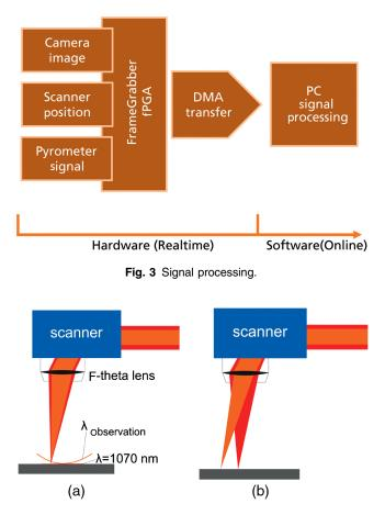
Fig. 4 Axial (a) and lateral (b) chromatic aberrations in f-theta lenses.
