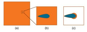
Fig. 1 Strategies for process observation: full-scan field (a), spatially resolved interaction zone (b), focused on melt pool (c).
