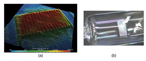
Fig. 10 Temperature map of filament (a) from halogen bulb (b).
