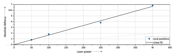
Fig. 8 Focal position depending on laser power.
