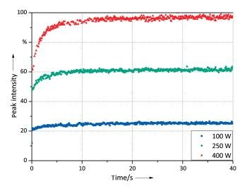
Fig. 9 Transient behavior of optical system for different laser powers.
