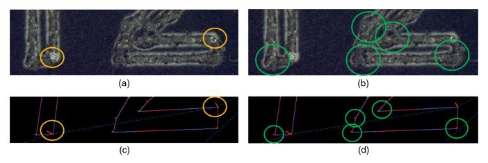
**Fig. 13** Microscope image of an aluminum sample with remolten spots (a, b) and plot of the number of same positions per unit time (c, d). (a, c) Image with orange circles shows start and end point of the contour, (b, d) image with green circles shows the corners.
