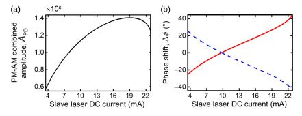
**Fig. 5** (a) Simulation results of the amplitude of the PM–AM combined signal as a function of the slave laser DC current. (b) Phase shift  $\Delta \phi (= \phi_{ML} - \phi_{OL})$  as a function of the slave laser DC current using the AM compensation method. Both the red solid and blue dashed curves are potential solutions.
