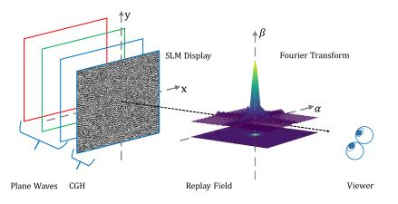
Fig. 1 A typical system for CGH consisting of three main components: a light source, a computer or hardware platform for interference pattern calculation, and a device to display the hologram.<sup>4</sup>
