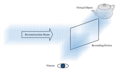
Fig. 4 A holographic projection system for hologram reconstruction.
