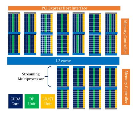
Fig. 5 A typical parallel pipeline overview of an NVIDIA GPU consisting of streaming multiprocessors each containing a number of cores and functional units.
