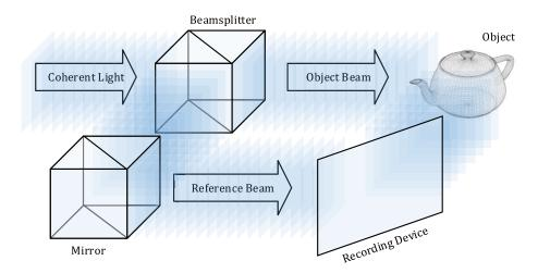
Fig. 3 A holographic imaging system for hologram recording.
