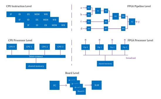
**Fig. 8** Different levels of parallelism and concurrency on hardware platforms. The left-hand side depicts the CPU instruction pipeline and processor-level parallelization, whereas the right-hand side shows the FPGA parallelization at the equivalent levels. Hardware clustering at the board level further exploits parallelism.
