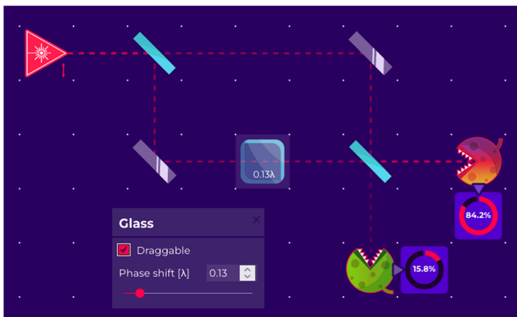
Fig. 15 Changing relative optical paths in the Mach–Zehnder interferometer. We use the high-intensity visualization mode.
