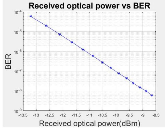
Figure 5. Received optical power vs BER
