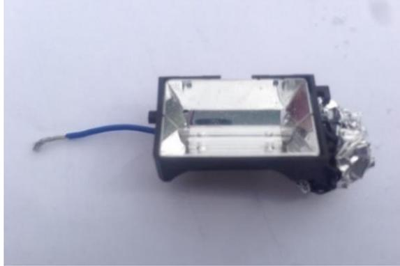
Figure 4. A static electricity detector using a camera's flash tube .
