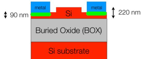
Figure 1. Cross section of the process. One can see the 90nm slab of silicon along with a 220nm thick waveguide. The N++ contact dopant is highlighted in green.
