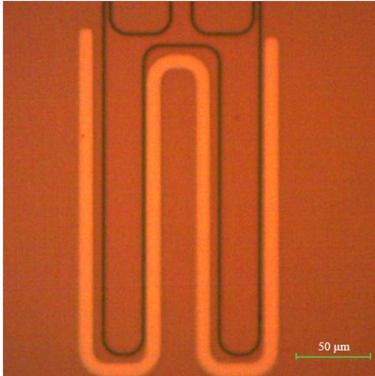
Figure 4. The chip after the oxide lift-off process. The light area is exposed silicon where the N++ dopant will diffuse. The darker area is the oxide mask.
