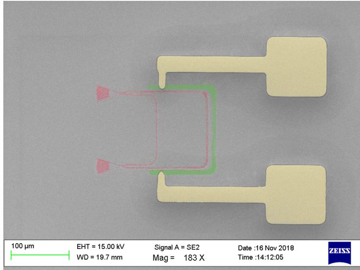
Figure 6. A false-color SEM image of an interferometer with the diffused N++ contact dopant and gold contact pads. The red area represents the silicon waveguides and grating couplers that make up the thermo-optic switch. The green area represents the N++ contact dopant. The gold area represents the gold contact pads.
