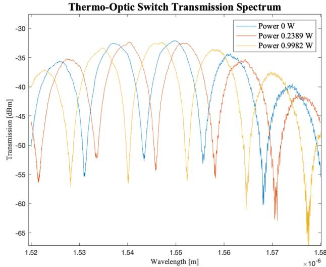
Figure 7. The transmission spectrum of one of the thermo-optic switches. The power consumption is high for a number of reasons. First, this measurement includes the contact pad resistance which is comparable to the heater resistance. The second major element is the 90nm silicon slab dissipates the heat away from the waveguide, wasting power. In the future, this can be easily eliminated by performing a second silicon etch to isolate the heater and waveguide from the remainder of the chip.
