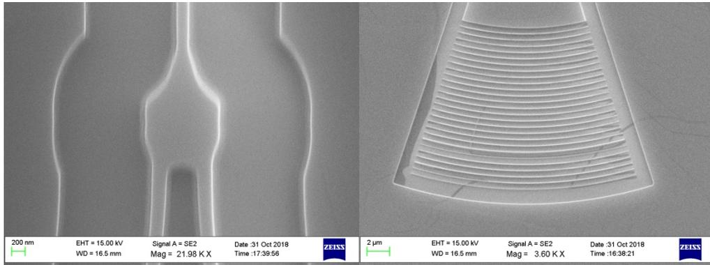
Figure 3. On the left is a y-splitter after the ECR etching process. These are used in the student designs to produce the interferometers used in the thermo-optic switches. On the Right is a grating coupler after the ECR etching process. These are used to couple light into the thermo-optic switches.
