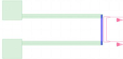
Figure 2. An example of a thermo-optic switch based on a Mach-Zehnder Interferometer. The waveguides that make up the interferometer are visible in red. The N++ contact dopant that forms the heater is visible in purple. The metal is visible in green.
