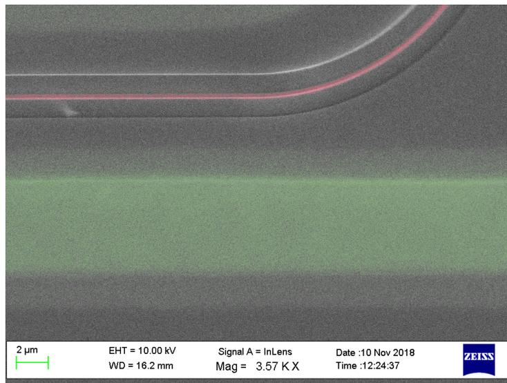
Figure 5. A false-color SEM image of an interferometer with the diffused N++ contact dopant. The N++ contact dopant is visible in green. The 220nm thick silicon waveguide is visible in red. The gray area represents a 90nm thick silicon slab.
