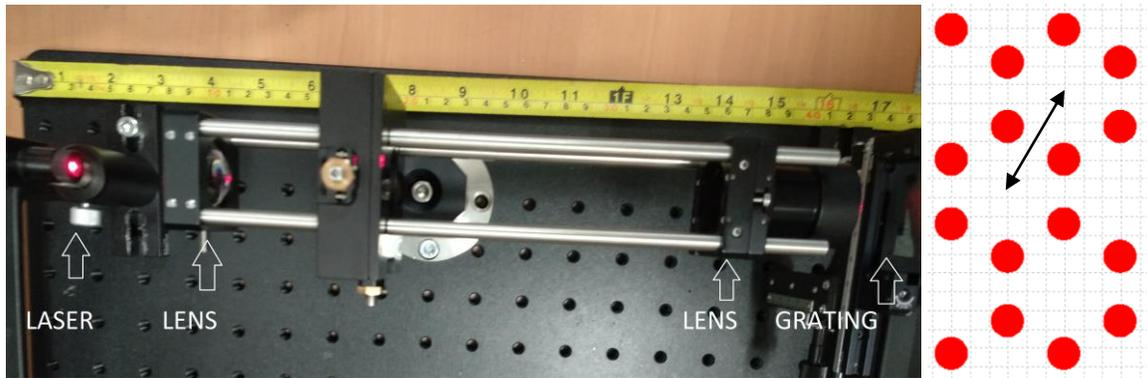
Figure 3. The beam is first expanded with a 2-lens telescope and then passes through the pattern. (One unit cell of the pattern used is shown to the right, where the red circles are open and the rest is opaque with chromium). The spacing between centers of the hexagonal array illustrated by the arrow is 0.72 mm and the radii of the red openings are 0.10 mm.
