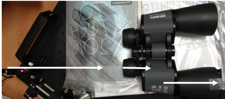
Figure 4. No optical table is necessary and no beam expander is necessary. In this case, a 12x50 binocular half acts as a beam expander.
