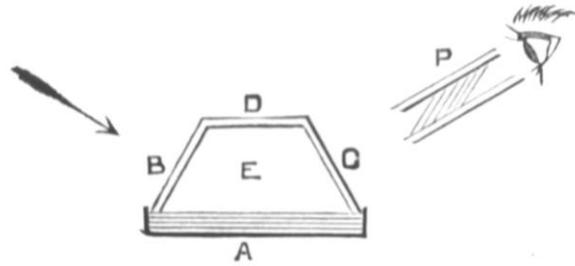
Figure 1. The stacked glass polariscope, reproduced from Ref. [20], Fig. 167. Understanding of this polarizer is slightly more difficult for students than other types of polarizers.
