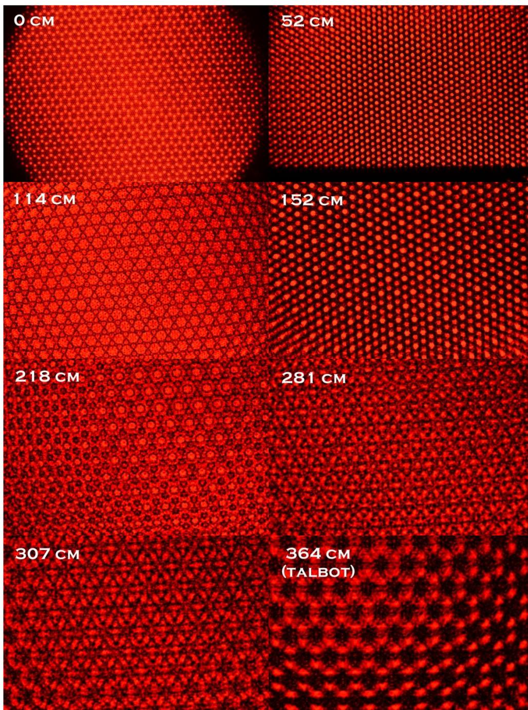
Figure 6. The diverging beam shows increasing magnification, and an increased distance to the Talbot image.
