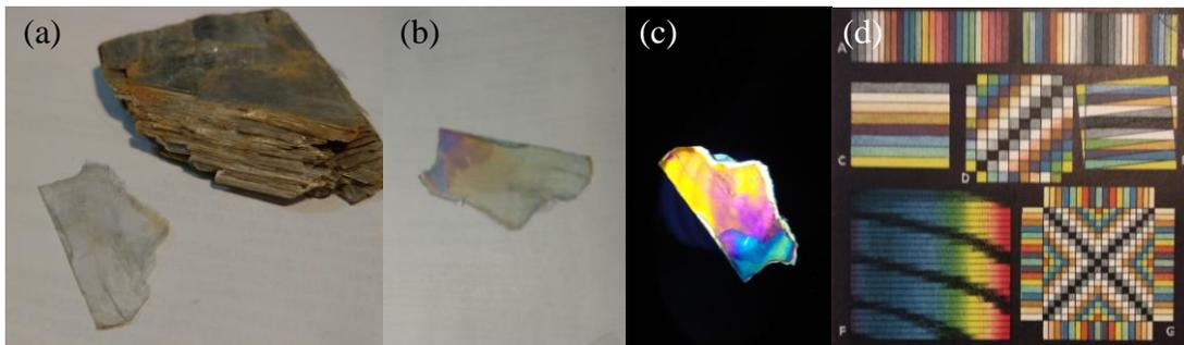
Figure 2. Experiment by the author: (a) A book of mica with one leaf cut away, (b) the leaf between parallel Polaroid pieces, (c) the leaf between crossed Polaroid pieces (illuminated from behind). (d) A similar setup with a more elaborate design in the 1892 reference [20].
