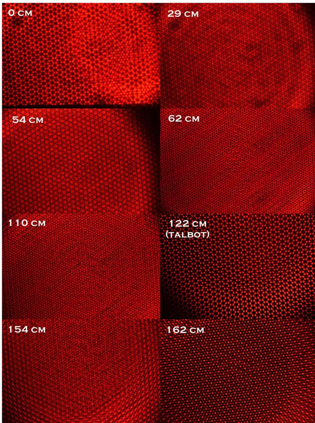
Figure 7. The aperture of the binoculars was more than twice the diameter of the expanded beam of the setup in Figure 5 resulting in improved images.
