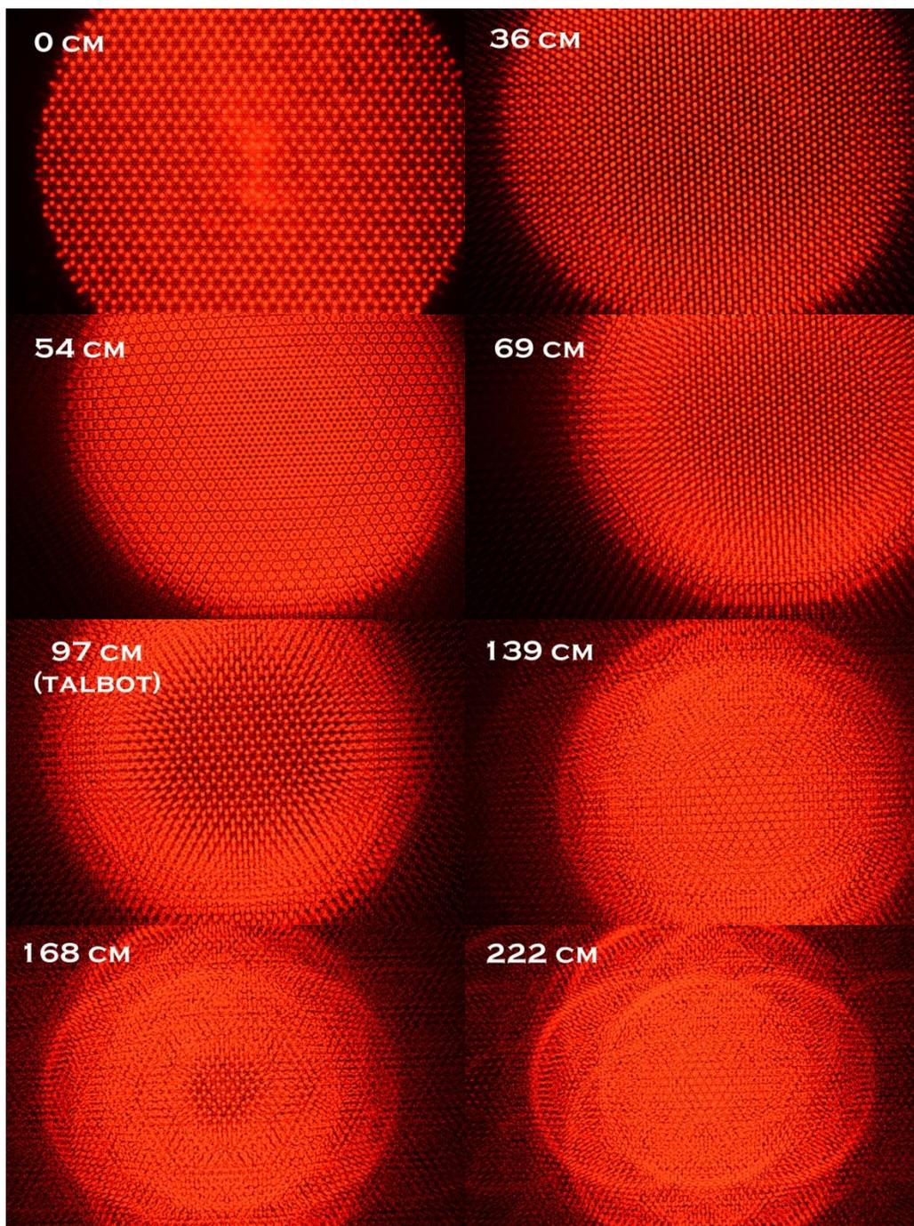
Figure 5. Direct observations at the image sensor with approximate distances from the grating marked with an expanded, collimated beam. Exact calculation of the Talbot distance for such a grating is described in detail in [48].
