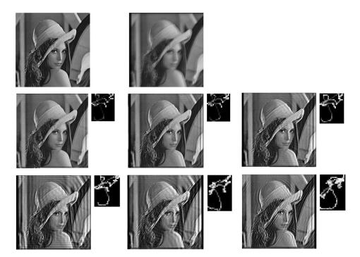
Fig. 8 Noise in gyroscope data. Synthetically blurred Lena image using PSF from recorded gyroscope samples and afterward deblurred using PSF from measurements with variable amount of noise. Images are from left to right, top to bottom: original, blurred, and six deblurred images using original gyroscope data altered by random Gaussian noise with variance from 0 to 0.05 (gyroscope measurements are in rad/s).
