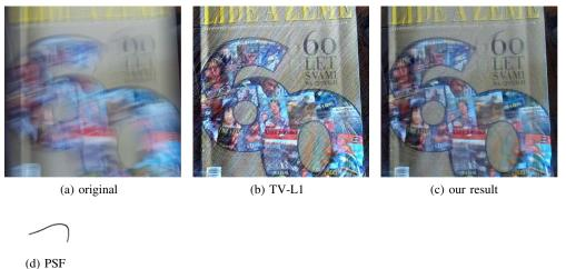
Fig. 4 Test 2: 1/9 s exposure, 21 × 28 estimated PSF.
