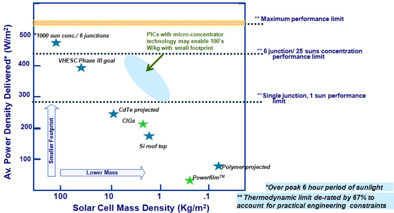
**Figure 4.** A plot of commercially available solar technology shows a trade-off between power density and mass density. It is envisioned that combining PIC technology and micro-concentration will enable PV performance that achieves unprecedented power-per-mass (blue oval) within a small footprint. The goal is to exploit the economies of scale for mass produced solar PV PICs and micro-optics to enable lower performance per cost than conventional PV panels may achieve.
