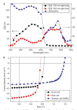
Figure 2 Quantum efficiencies, J–V characteristics and stability of single cells and tandem cells. a, EQEs of the inverted tandem solar cell and absorption spectrum (without metal electrode). b, J–V characteristics of the front cell, rear cell and inverted tandem solar cell, tested at NREL using the OSMSS simulator.
