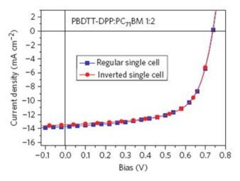
Figure 1. J–V characteristics of single-cell devices with regular and inverted structures under AM1.5G illumination from a calibrated solar simulator with an irradiation intensity of 100 mWcm<sup>2</sup>.
