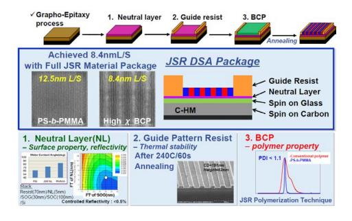
Figure 4. JSR's DSA BCP package and performance.
