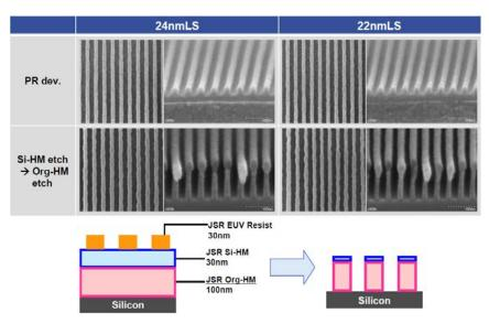
Figure 6. JSR's EUV hardmask package.
