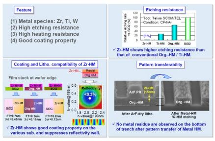
Figure 7. JSR's metal hardmask.
