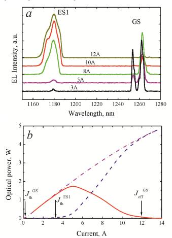
Figure 1. Lasing spectra at different currents (a); laser power (b): dashed-dotted curve – total (GS+ES1), solid curve – ground-state component (GS), dashed curve – first excited-state component (ES1).
