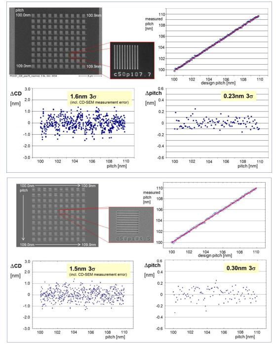
Figure 7: eMET POC exposure of 50nm lines whose pitch was varied between 100.0nm and 109.9nm in 0.1nm steps; vertical lines in HSQ negative resist and horizontal lines in pCAR positive resist. The line width and pitch values are written with 30nm line width.
