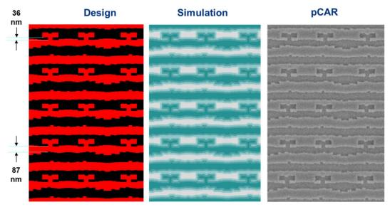
Figure 12: eMET POC exposure of aggressive OPC mask pattern in pCAR positive resist.
