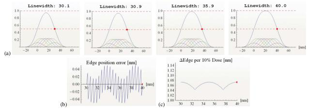
Figure 6: (a) Simulated change of edge position in 0.1nm steps showing several examples between 30.0nm and 40.0nm; (b) Simulated deviation of edge position from 0.1nm address grid; (c) Simulated change of edge with 10% change of dose vs. line width.
