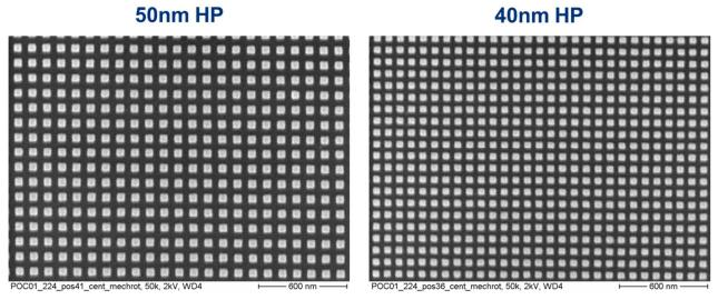
Figure 9: eMET POC exposure of 50nm HP dots and 40nm HP dots in HSQ negative resist with improved corner rounding.
