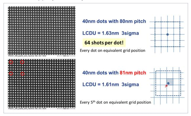
Figure 8: eMET POC exposure of 40nm dots in HSQ negative resist with 80nm pitch (above) and 81nm pitch (below).
