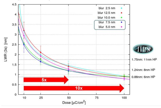
Figure 15: Monte Carlo simulation of the 3sigma line width roughness (LWR) for 30nm line width vs. resist exposure dose. Parameter is the combined tool and resist 1sigma blur. The optimum total 1sigma blur is between 5nm and 7.5nm, meeting the requirements for the 6nm HP mask technology node when using a resist exposure dose of  $100\mu$ C/cm<sup>2</sup>.
