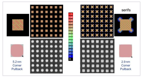
Figure 10: Bit map (above) and 50nm HP dot exposure (below) in HSQ negative resist without (left) and with (right) improved corner.
