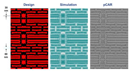
Figure 11: eMET POC exposure of aggressive OPC mask pattern in pCAR positive resist.
