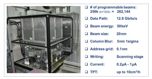
Figure 5: eMET POC during factory acceptance tests at IMS Nanofabrication, Vienna, Austria and main specifications.
