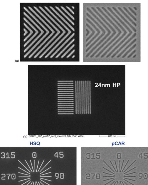
135 225 80 (c) POC01 291 pos102 700 nm POC01\_292\_pos055 - 700 nm Figure 14: eMET POC resolution (a) 45° and 135° 30nm HP in HSQ negative (left) and pCAR positive resist (right),
