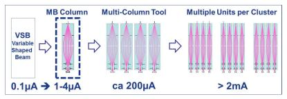
Figure 2: Evolution of electron beam systems as needed to realize 100WPH EBDW
