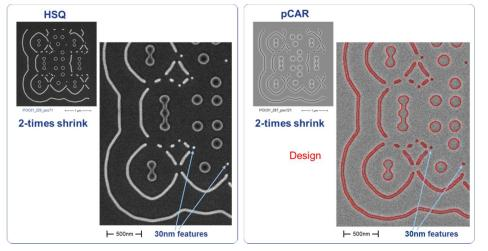
Figure 13: eMET POC exposure of ILT mask pattern in HSQ negative and pCAR positive resist. The ILT test pattern was provided by DNP [18, 19] and was exposed according to design and also with 2-times shrink.
