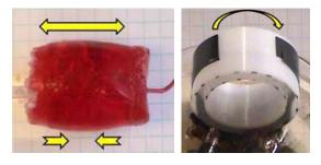
Picatinny Arsenal, NJ, United States, presented "Electrically Driven Mechanochemical Actuators". Using Carbon infused contractile EAP, a demonstration has been made showing an electrically driven mechano-chemical actuators performing rotational and push-pull
