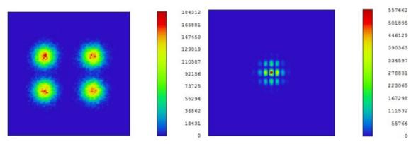
**Figure 3** - Coherent beam combining of a 2x2 laser array in Zemax. The 4 individual elements are shown on the left and then when combined the central peak is intensified and the sidelobes suppressed. With additional elements the peak will grow and the sidelobes will decrease. Our baseline uses a filled close packed array to minimize sidelobes and to maximize the central peak.
