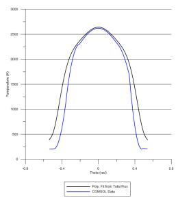
Figure 12 - Comparison of 2 and 3 D models temperature vs. theta (angle from beam axis on sphere) for SiO<sub>2</sub> with 50GW total power and sigma =5m Gaussian beam illumination. Results are nearly identical in the critical central region.
