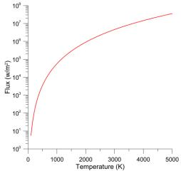
**Figure 7-** Relationship between flux and temperature in spot in the radiation dominated case. In reality the temperature rarely gets above 3.000K as power in diverted from radiation to mass ejection.
