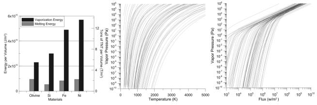
**Figure 4 - Left:** Melting and Vaporization energy per unit volume for S type (Si rich) asteroids. **Middle:** Vapor pressure vs. T for virtually all elements on the periodic table (93 are modeled). **Right:** Vapor pressure vs. target flux for the same 93 elements. The upper outlier is Mercury.
