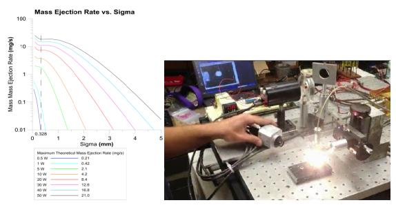
Figure 14 - Left: 2D simulation with laboratory test parameters. Similar to Figure 7 but set for lab testing. Plot is of expected mass ejection vs. sigma (Gaussian beam) for various power levels. Measured sigma based on hole size in targets is less than 330μm. Sample is assumed to be SiO<sub>2</sub>. Right: Video 1:http://dx.doi.org/10.1117/12.2030228.1Picture of test system. Small camera is an 8-12 micron FLIR IR microbolometer unit. Sample is sand.
