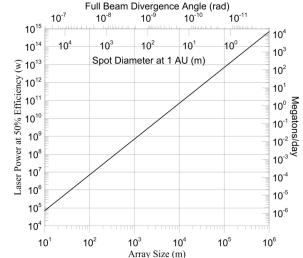
Figure 2 - DE-STAR laser power, diffraction limited beam divergence and spot size at target engagement of 1AU.
