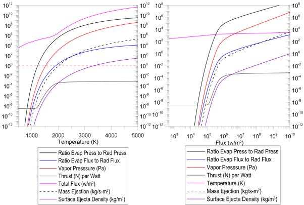
Figure 9 - Left: Simulations of SiO<sub>2</sub> properties vs. temperature. Right: Simulations of SiO<sub>2</sub> properties vs. flux.
