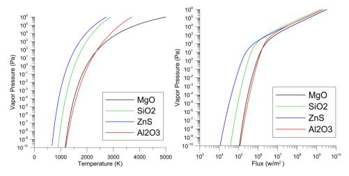
**Figure 5 - Left:** Vapor pressure vs. T for four common high temperature asteroid compounds. **Right:** Vapor pressure vs. target flux for the same found compounds. Note that at temperatures of 2,000-3,000K or fluxes of about 10MW/m<sup>2</sup> the vapor pressure and hence mass ejection rates are very high.
