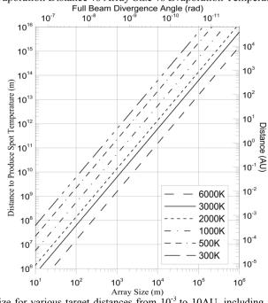
Figure 6 - Left: Spot temperature vs. DE-STAR array size for various target distances from 10<sup>-3</sup> to 10AU, including average solar illumination on asteroid (sets lower limit on asteroid or comet temperature). Right: Distance to target vs. array size for various spot temperatures from 300-6,000K. At 300K icy comets become targets while at 6,000K (hotter than sun) no known material survives.
