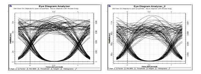
Figure 8 Eye diagram of Complementary technique at (155 Mb/s) for 30 km distance
