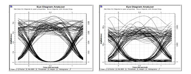
Figure 5 Eye diagram of NAND subtraction technique at (622 Mb/s) for 30 km distance
