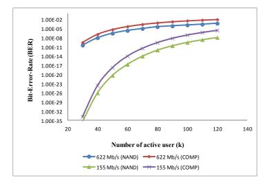
Figure 2 BER versus number of active users against different bit rate
