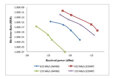
Figure 9 Received power versus BER for both techniques
