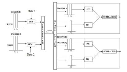
Figure 1 Implementation of NAND subtraction technique
