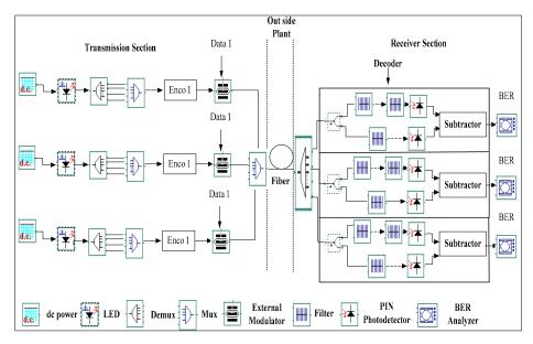
Figure 3 Simulation setup for OCDMA system using NAND technique with EDW code
