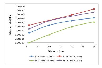
Figure 4 BER versus distance using NAND and Complementary technique at various bit rates for EDW code.
