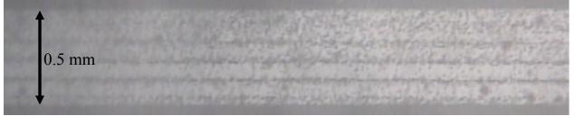
Figure 7: 6 µm particles concentrated at the nodes of standing waves in water in a PDMS channel on 128° Y-cut black lithium niobate with a 200 µm wavelength IDT pair driven at a frequency of 19.76 MHz
