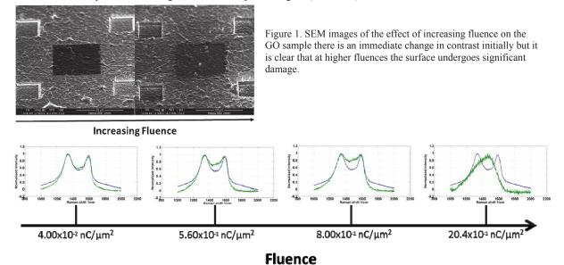
Figure 2. Optical images of the exposed regions with their corresponding Raman spectra, these results show us that the sample initially undergoes reduction and then at higher ion fluences amorphisation.
