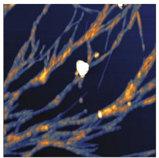
Figure 1 ac- $\beta L\beta I\beta A$  on mica surface, imaged by AFM. The scale is 10  $\mu$ m. The peptide was dissolved in methanol and mixed with isopropanol for deposition. Typical heights of fibres are 20-30 nm
