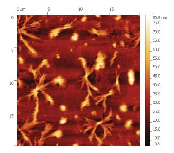
Figure 2 Peptides were deposited from methanol with an addition of isopropanol. Self-assembly was aborted via quick drying. The nucleation sites of fibre formation are visible as radial structures.
