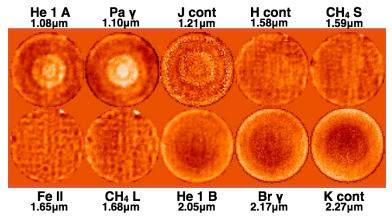
Figure 4. Center phase maps extracted from data taken at various narrow- and medium-band filters available on NIRC2. There is a visible apparent focus offset.
