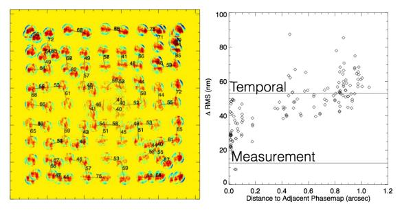
Figure 3. Grid of adjacent phase maps and the associated wavefront error between the adjacent samples.
