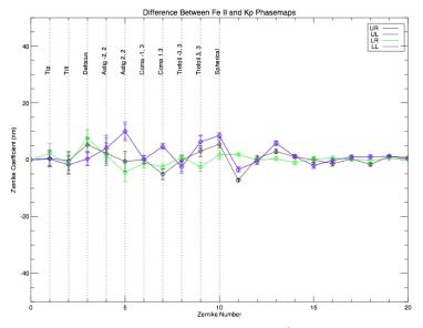
Figure 7. Zernike decomposition of the optical path differences between K' and Fe II at positions fairly close to the center of the detector that stayed in the 320  $\times$  312 subarray of the detector. The lower-order terms again dominate the overall wavefront error.
