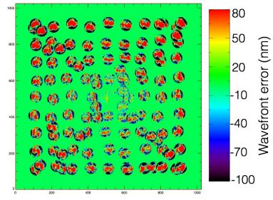
Figure 2. Our full phase diversity data grid, where phase diversity data is taken at various points across the field of view. There are 150 different data sets (some taken at the same position to study time variability affects). All data is taken through the Fe II narrow-band filter on NIRC2 ( $\lambda_0 = 1.65 \ \mu m$ ).
