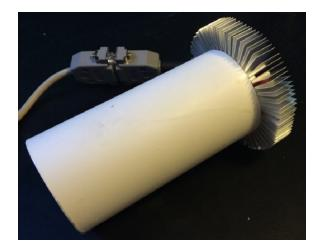
Figure 3. The light engine with the mixing tube.
