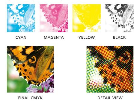
Figure 13. The typical CYMK printing process and the resulting dot patterns. [15]
