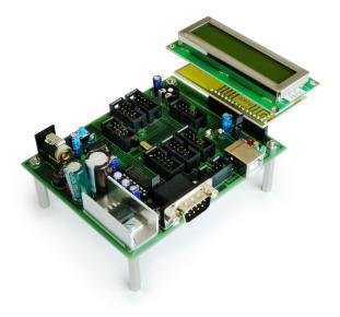
Figure 1: Microcontroller board with display
