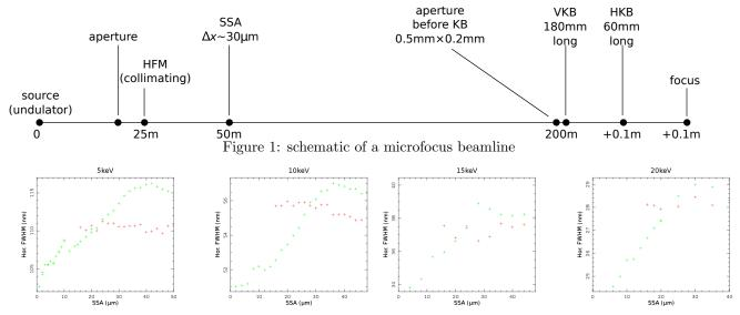
Figure 2: Horizontal focus size, red - single electron calculation, green - multi-electron calculation (20000 electrons)
