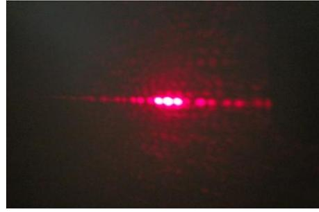
Fig. 6: Slits with 0.2mm width
