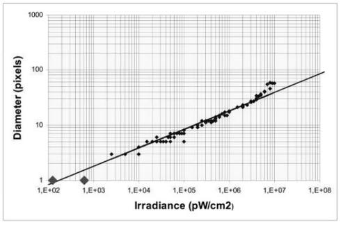
Figure 8 Spot size vs. laser power
