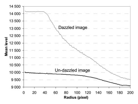
Figure 6 Dazzle energy vs. radial distance
