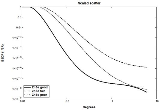
Figure 4 Bi-directional Scatter Distribution Function
