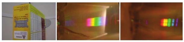
Figure 2. Workshop-made spectrometer (left), built following instructions from Dr. Andrew Steele (University of Oxford), and spectra of conventional (center) or efficient (right) light bulbs.
