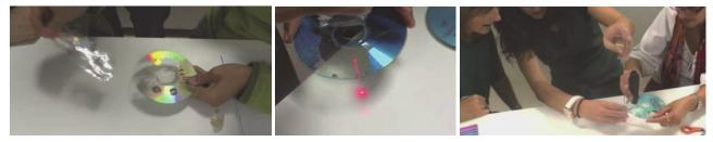
Figure 1. Participants in a teacher training workshop peel off the reflecting layer, study the diffraction phenomenon and perform the measurements needed in order to calculate the grating period.
