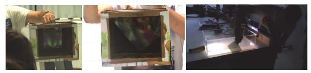
Figure 5. Polarization experiments: visualization of the mechanical tensions in a CD plastic case with a polariscope (left), illustration of the birefringence properties of an acetate transparency acting as a half-wave plate (center), and study of the polarization of scattered light (right).
