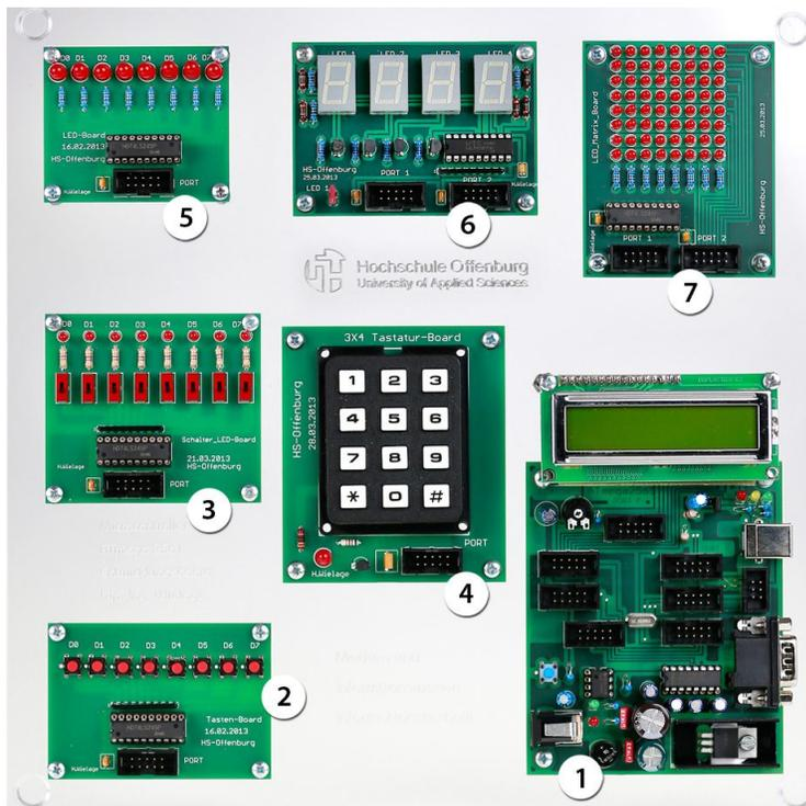
The development board is structured modularly. At the bottom right you find the microcontroller board with its LCD (1).
