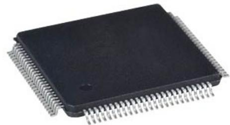
Figure 1: Microcontroller “ATMEGA 2561” [2]
