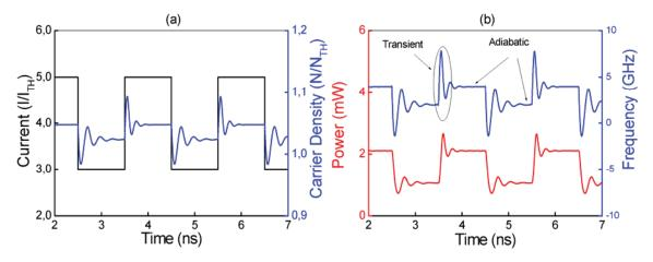
Figure 3. Results obtained with the rectangular current waveform selected, bias set to 4  $I_{TH}$ , amplitude 2  $I_{TH}$  and frequency 0.5 GHz: (a) current and carrier density, black line left axis and blue line right axis, respectively and (b) output power and chirp, red line left axis and blue line right axis, respectively.
