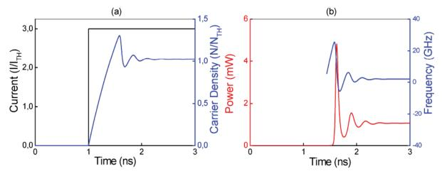
Figure 2. Results obtained with the rectangular current waveform selected, bias set to 0 and amplitude 3 ITH: (a) current and carrier density, black line left axis and blue line right axis, respectively and (b) output power and chirp, red line left axis and blue line right axis, respectively. The time axis is zoomed 3 ns around the laser switch on.
