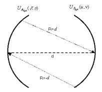
Figure 2. Fresnel diffraction between the spherical surfaces
