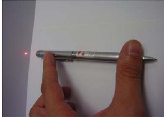
Figure 3. Laser pointer used for obtaining the holograms
