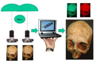
Figure 6. Representation of the necessary steps for obtaining anaglyphs
